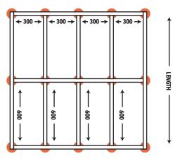
Please make sure that if you are joining joists together to create a longer length, that all joints are supported with a timber post or decking pedestal. (for example 2 joists at 3m to create a 6m span, this would need supporting in the centre where the two joists meet)
